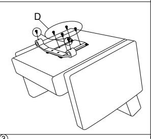
Attach the footrest bar to the front pair of holes in the chair bracket using the remaining 2 bolt sets removed in step 1.
